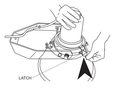
Figure 12. Securing Latch
